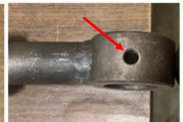
Modified Turnbuckle (right) Grease nipple added
