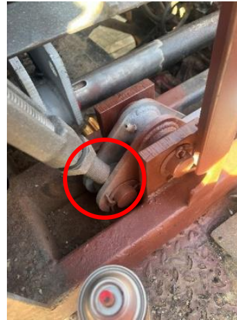
The location where the brake turnbuckle parted from the rig structure.
